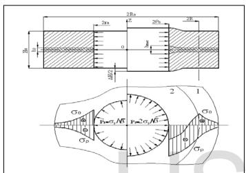
Fig. 1. represented the initial (left) and final (right) shape and dimensions of the unit, as well as the stress distribution at the initial and the limiting value of internal pressure (1-elastic region, 2-plastic region).
